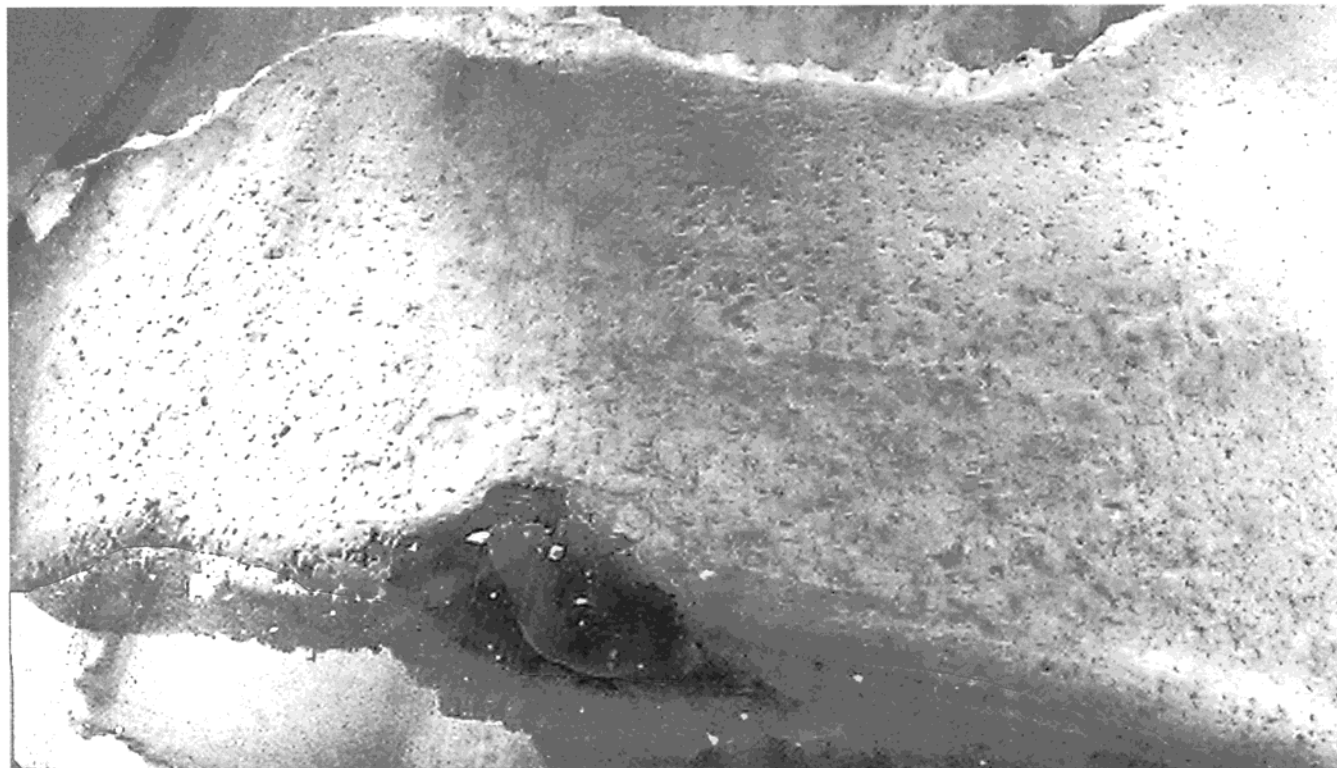
Figure 1. Image showing the polynorbornenamer obtained directly from ROMP in scCO_2 as described in entry 5 of Table 1. The dark spot containing the metal species is clearly visible within the white bulk polymer.
